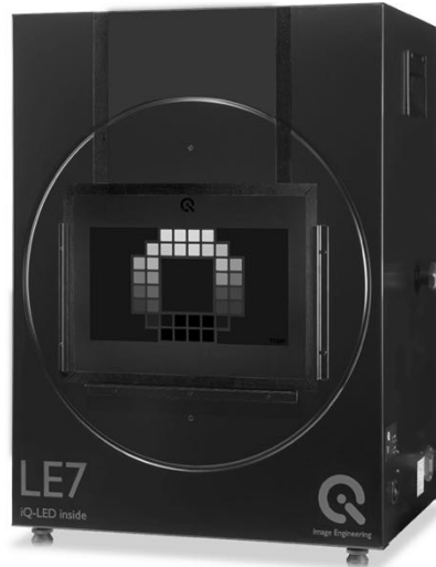
< The TE269 test target with the LE7 illumination device (integrating sphere) >
