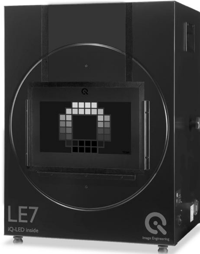
< The LE7 uniform light box with the TE269 OECF test chart >
